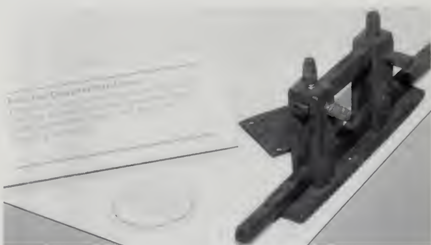
Fig. 7. The "Settlement" exhibit, Michigan Historical Museum, Lansing, MI. The actual die is an engraved steel plate, which can be seen behind the "tool". Holes in the plate were used to hold it in place in the tool while it was struck, probably with a heavy hammer. The round "blob" seen in the foreground of the photo, to the left of the tool, is a wax impression of the die, which is dated 1832.
