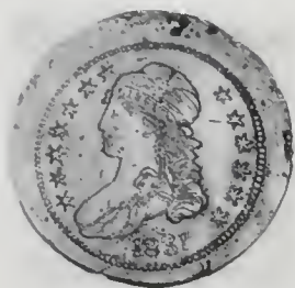
Fig. 36. Uniface counterfeit 1831 obverse die trial on lead "slug".
