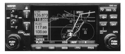
Figure 2-3. The GNS 430 is a GPS/VHF nav-comm unit.
