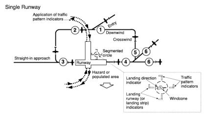
Figure 4-2. Traffic pattern, single runway (from AC 90-66A)
