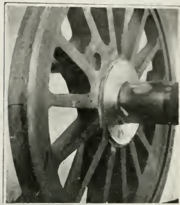
Fig. 3. Finished Hub Liner.
