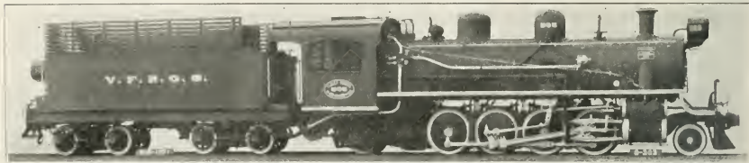
Mikado Locomotive, Rio Grande do Sul State Railways, Brazil, built by Montreal Locomotive Works.
