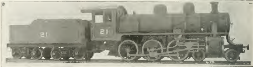
Ten-wheel Locomotive, for Trinidad Government Railways, built by Montreal Locomotive Works.
