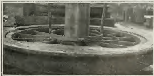
Fig. 2. Pouring Hub Liners. Wheels on End, Ready for Pouring.
