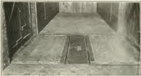
60-Ton Hopper Bottom Box Car, C.P.R. Interior, with hopper closed. See article on page 25.
