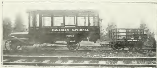
Gasoline Driven Motor Passenger Car and Baggage Trailer, on Canadian National Railways, Stanley Subdivision, New Brunswick.
