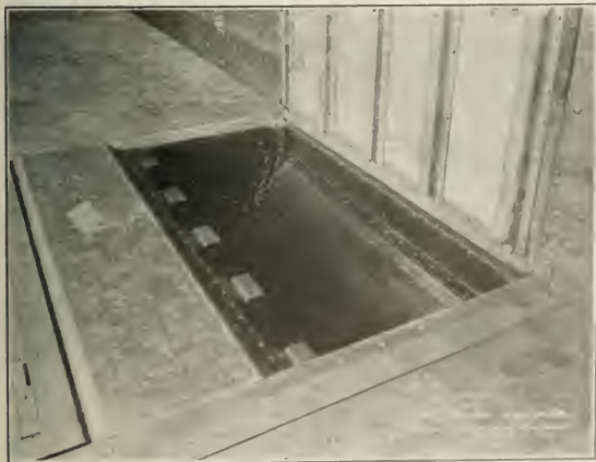
60-Ton Hopper Bottom Box Car, C.P.R. Floor section raised for grain loading. See article on page 25.
