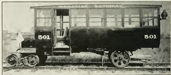
Gasoline Passenger Motor Car, on trial on Canadian National Railways.
