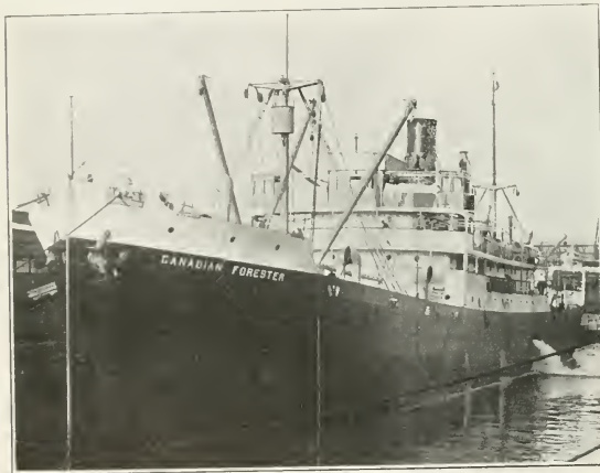
Steel Cargo and Passenger Steamship, Canadian Forester, approximately 5,100 d.w. tons, built for Canadian Government Merchant Marine by Tidewater Shipbuilders Ltd.
