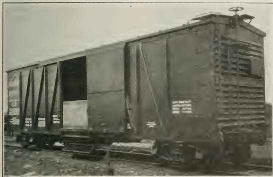
60-Ton Hopper Bottom Box Car, C.P.R. Hopper door open.
