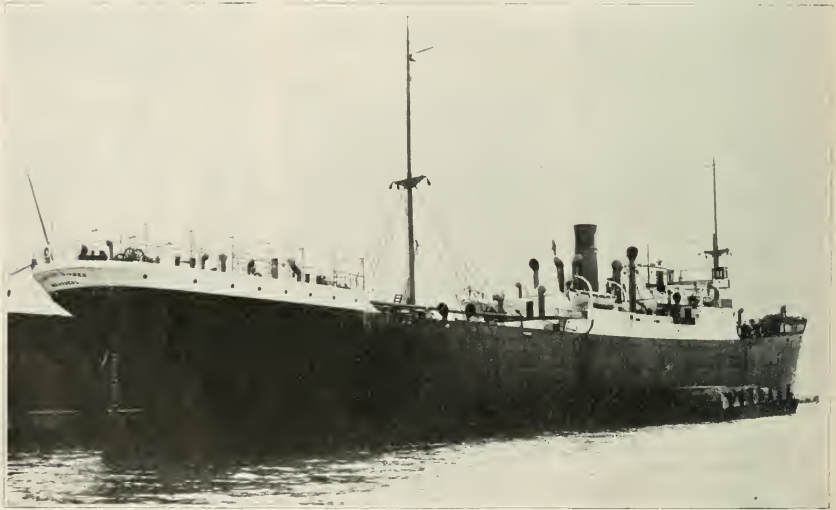
Steel cargo steamship Canadian Winner, approximately 8,390 d.w. tons, built for Canadian Government Merchant Marine Ltd., by Harbour Marine Co., Victoria, B.C.
