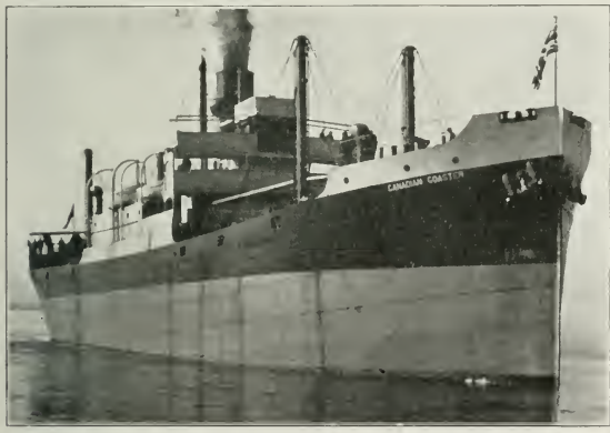
Steel Cargo Steamship Canadian Conster, approximately 3,890 d.w. tons, built for Canadian Government Merchant Marine, by Collingwood Shipbuilding Co., Kingston, Ont.
