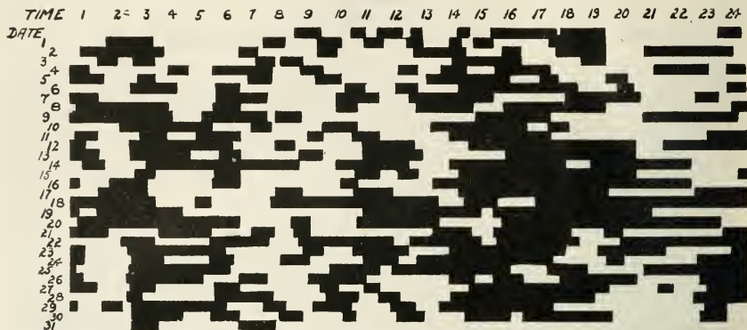
Smoke Chart, Connaught Tunnel, C.P.R., for March 1920. Clear intervals of less than 10 minutes are disregarded.
